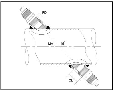
Figure 155: Determining the Pipe Coupling Length
